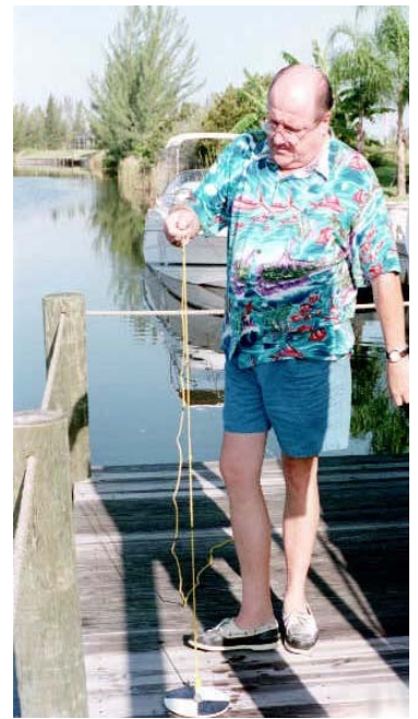
Joe Hauck measures the clarity of his canal with a Secchi disk.
